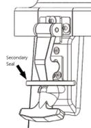
The rubber latch design allows the use of a zip tie, vet seal, safety seal, etc. to ensure integrity of product shipped.
